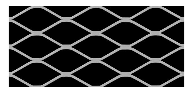
LW Aperture:43.43mmStrand Width:2.31mmSW Aperture:18.03mmThickness:1.14mmWeight:0.63 kg / m2Open Area:80%
